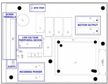
Figure 2 - Connector Layout
