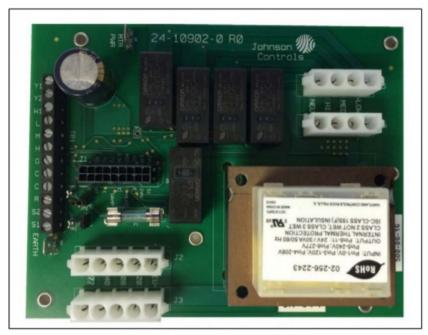
Figure 1- Fan Relay Board (FRBii)
