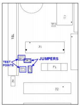
Figure F.2 - FRBii Jumpers and Test Points
